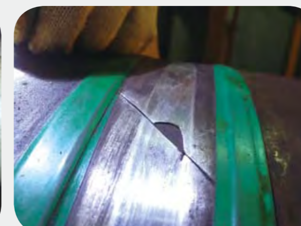
Faulty slip ring
