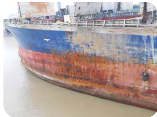
Hull conditions with defective ICCP system
