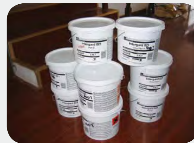
Epoxy filler for ICCP Di-electric shield
